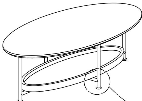
To adjust the adjustable leveler. If there is a gap between a leg and the floor, please adjust the adjustable leveler up or down under each leg.
