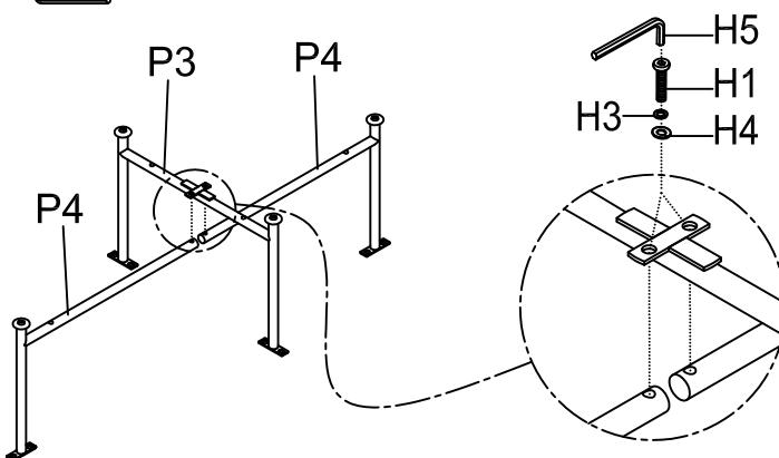
Step 2: Loosely attach Tray (P2) to Metal Leg A (P3) and Metal Legs B (P4) as shown below.
