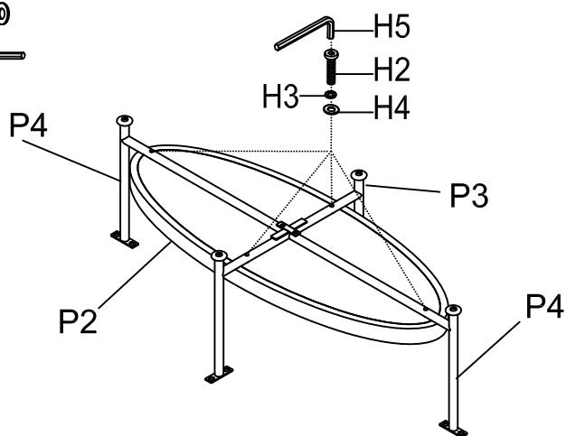
Step 3: Attach Metal Leg A (P3) and Metal Legs B (P4) to Table Top (P1) as shown below.
