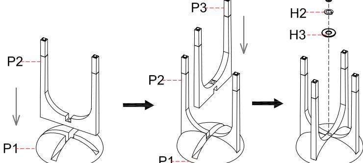
Step 2. Securely tighten the bolt with Allen wrench(H4), make sure the table is leveled and aligned properly. Turn the assembled table to an upright position. Assembly is complete. **Failure to follow these instructions may cause the bolts to misalign during assembly.**
