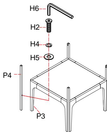
Step 3. Attach the top frame (P1) to the assembled metal legs (P4) as shown below.
