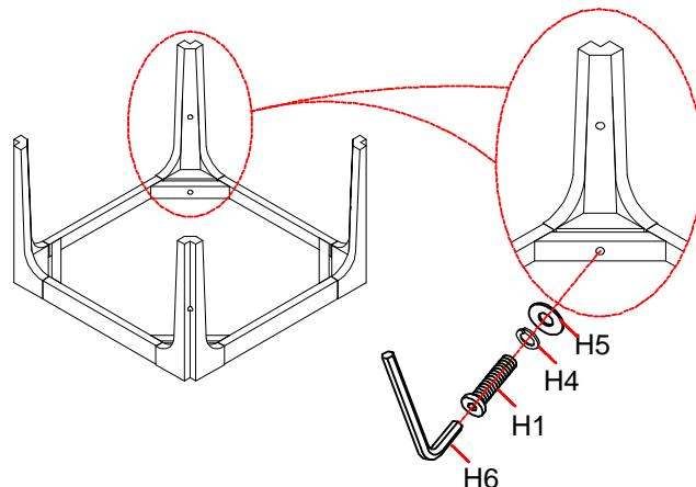
Step 2. Attach the metal legs (P4) to the wood legs (P3) as shown below.
