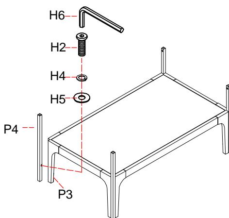
Step 3. Attach the top frame (P1) to the assembled metal legs (P4) as shown below.
