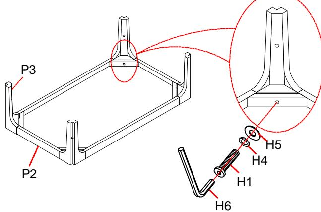
Step 2. Loosely attach the metal leg (P4) to the wood legs (P3) as shown below.
