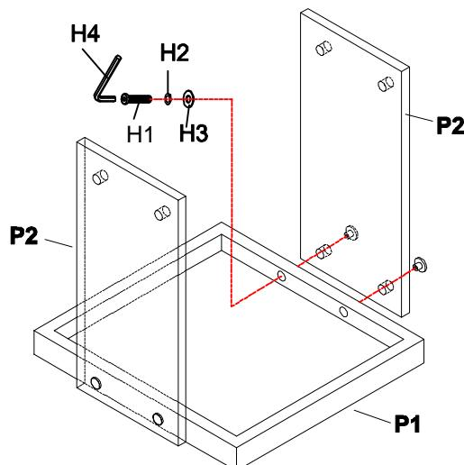
**Step 2.** Loosely attach bottom panel (P1) between two side panels (P2) using short Bolts (H1), lock washers (H2) and flat washers (H3) as shown below.
