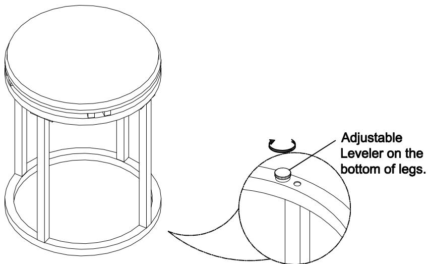
ADDITIONAL NOTE ABOUT SAFETY: BOLTS MAY LOOSEN DURING NORMAL EVERYDAY USE. THEY SHOULD BE PERIODICALLY INSPECTED AND RE-TIGHTENED TO PREVENT DAMAGE OR INJURY. ALWAYS CHECK TO BE SURE THAT ALL HARDWARE IS KEPT TIGHTENED.
