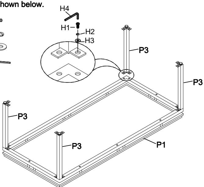
**Step 2.** Loosely attach the bottom frame (P2) to the legs (P3) using bolts (H1), lock washers (H2) and flat washers (H3) as shown below.
