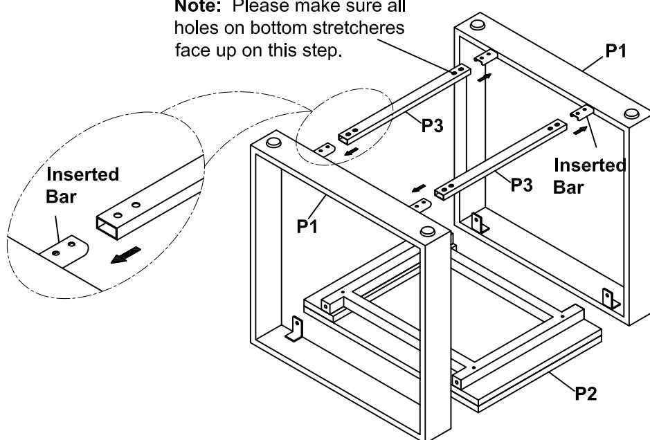
**Step 2.** Loosely attach side frames (P1) to the table top (P2) and bottom stretchers (P3) using bolts(H1&H2), lock washers (H3) and flat washers (H4) as shown below.
