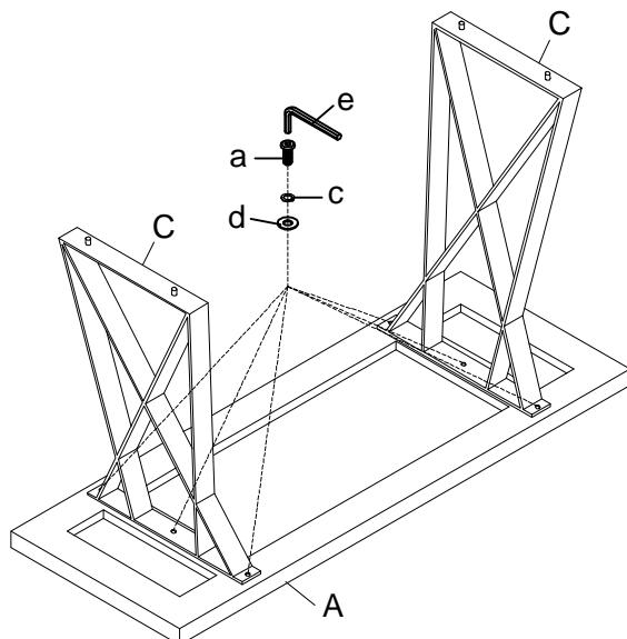
Step 2. Loosely attach the bottom panel (B) to assembled side frames (C) as shown below. Securely tighten all bolts with Allen wrench (e).
