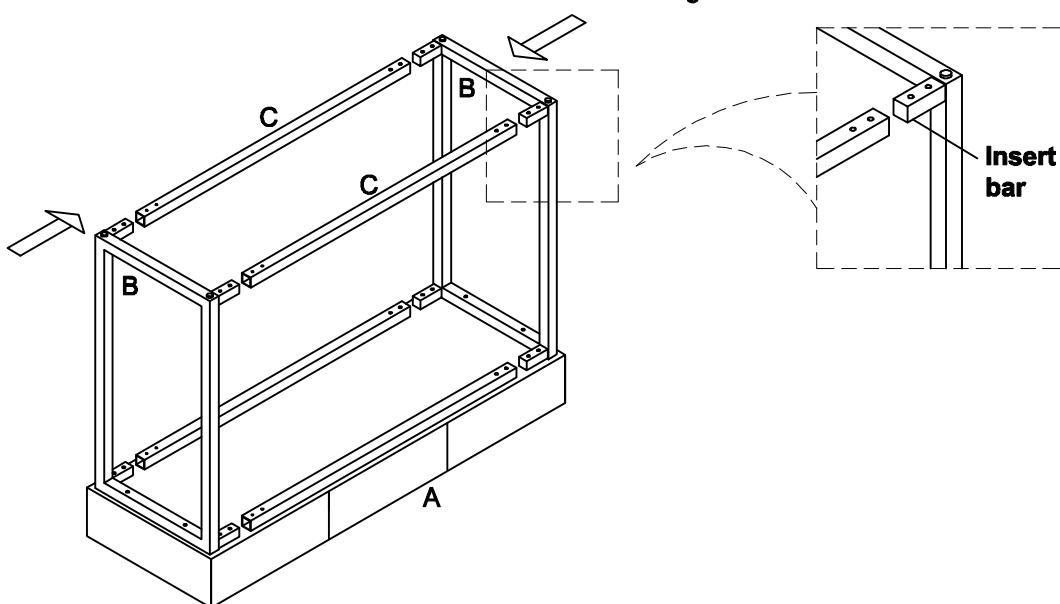
Step 2. Loosely screw all bolts (a & b) to side frames (B) to rails (C) and table top (A) as shown below by hand at first, then securely tighten all bolts with Allen wrench (e).
