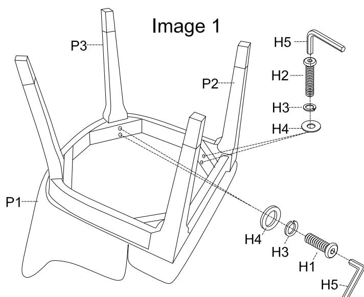
**ADDITIONAL NOTE ABOUT SAFETY: BOLTS MAY LOOSEN DURING NORMAL EVERYDAY USE. THEY SHOULD BE PERIODICALLY INSPECTED AND RE-TIGHTENED TO PREVENT DAMAGE OR INJURY. ALWAYS CHECK TO ENSURE THAT ALL HARDWARE IS KEPT TIGHTENED.**
