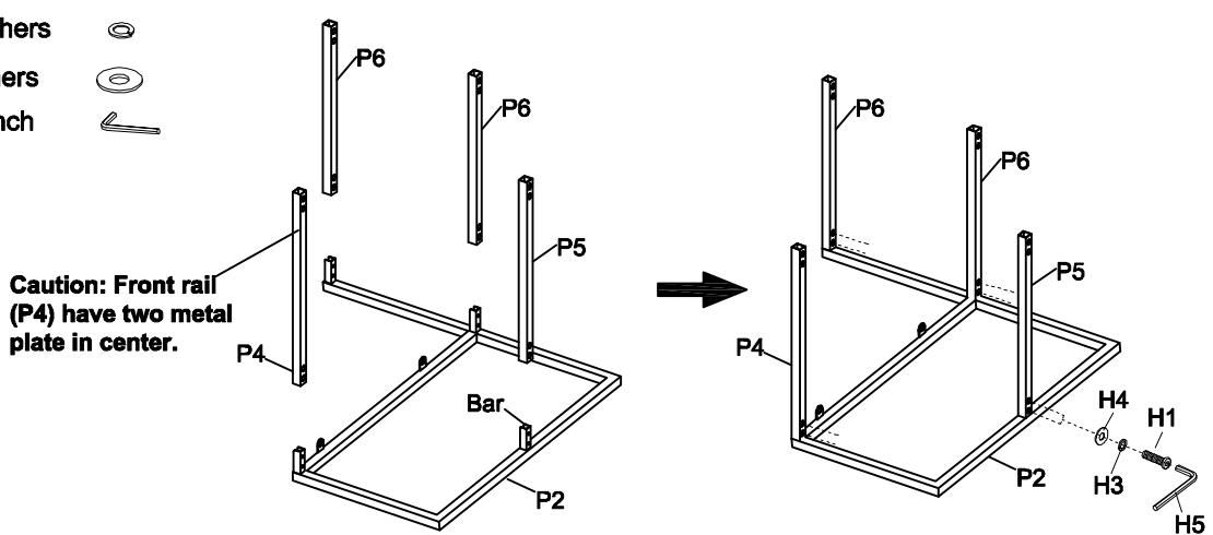
**Step 2. Attach the right side frame (P3) to the assembled each rail (P4,P5,P6) as shown below.**
