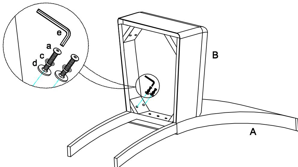
Step 3. Attach front legs (C) to seat cushion (B) using bolts (b), lock washers (c) and flat washers (d). Loosely tighten by Allen wrench (e).
