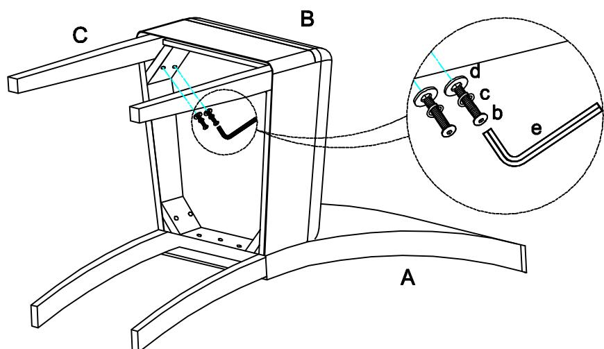
Step 4. Securely tighten all bolts by allen wrench (f). Assembly is complete.
