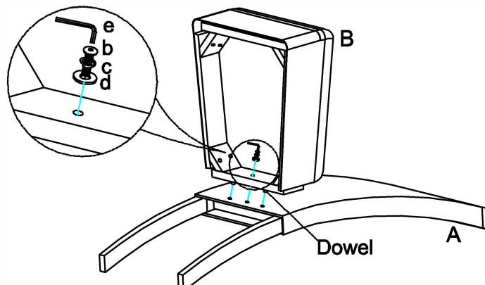
Step 2. Attach the seat cushion (B) to the leg of Chair back (A) using bolts (a), lock washers (c), flat washers (d). Loosely tighten by Allen wrench (e).
