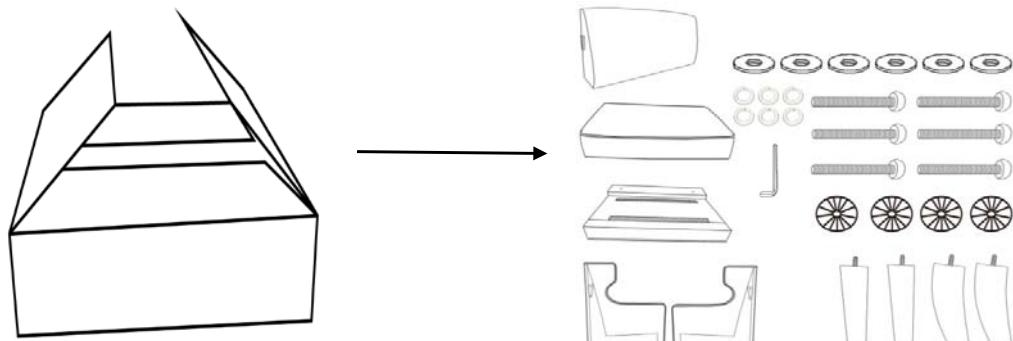
2. Open the black fabric under the seat frame. Align the holes on the seat frame(P4) and backrest(P5), by using flat washers (H3), lock washers(H2) and bolts (H1). Securely tighten all bolts with allen wrench (H4).
