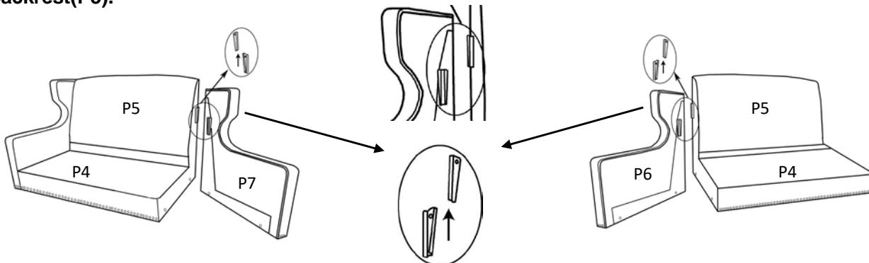
4. Align the holes on the seat frame(P4) and the arms(P6&P7),then using flat washers (H3), lock washers(H2) and bolts (H1). Securely tighten all bolts with allen wrench (H4).Close the black fabric with zipper.
