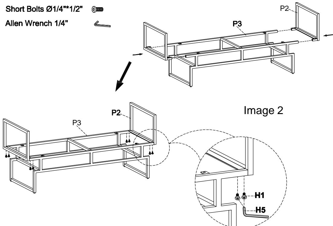
Step 2. Attach the assembled frame to the bottom of seat cushion (P1) as shown below image 3, securely tighten all bolts with Allen wrench(H5), make sure the bench is leveled and aligned properly. Turn the assembled bench to an upright position. Assembly is complete. **Failure to follow these instructions may cause the bolts to misalign during assembly.**
