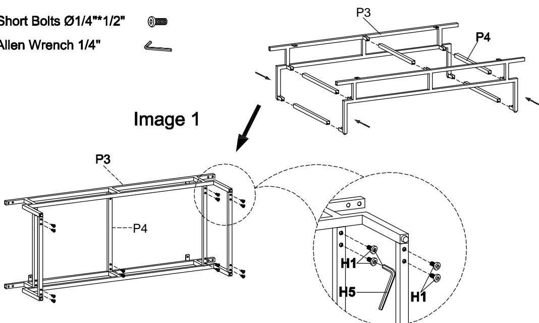
Step 2. Insert the side frame (P2) to the assembled front and back frame (P3) as shown below image 2.
