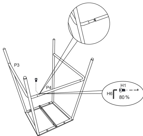
Step 4. Fully tighten bolts(H2 and H1) with allen wrench(H6) as illustration below.
