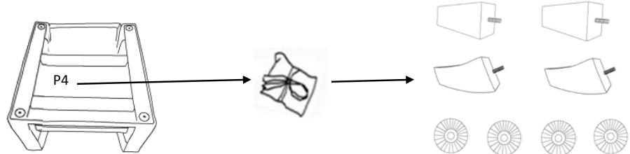
2. Place washers(H1) on legs(P1,P2) and attach to base by screwing clockwise into corresponding holes.
