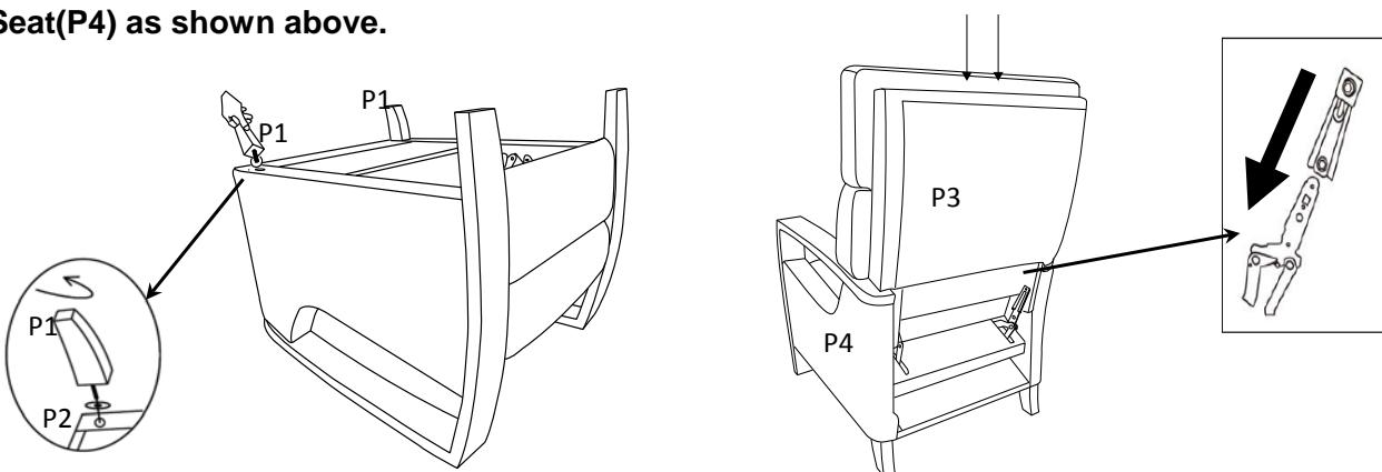
3. Smooth down the fabric flap on the Chair Backrest. Run your hands down both sides of the flap, from top to bottom, allowing the velcro tape to adhere to the flap under the seat of the chair.
