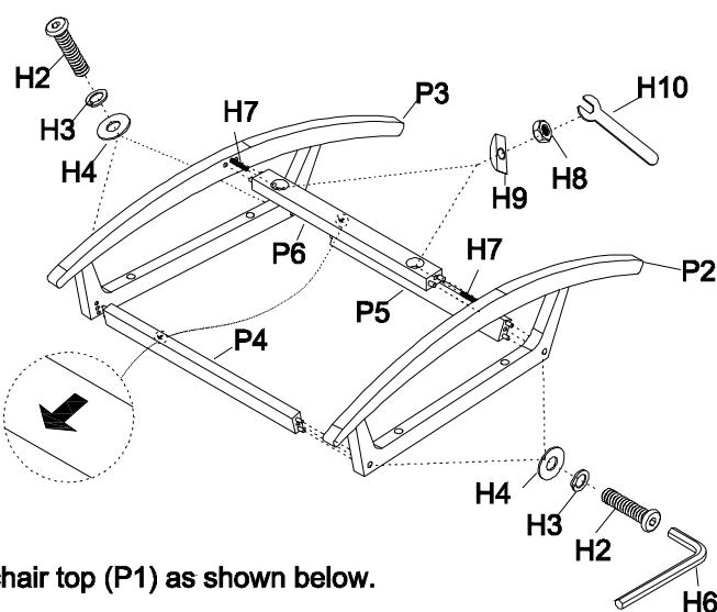
Step 2. Attach the assembled side frame to the chair top (P1) as shown below.
