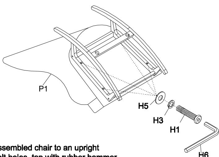
Step 3. Securely tighten all bolts, turn the assembled chair to an upright position. Insert wood plugs (H11) into the bolt holes, tap with rubber hammer or mallet until the wood plug edge are even with wood surface.
