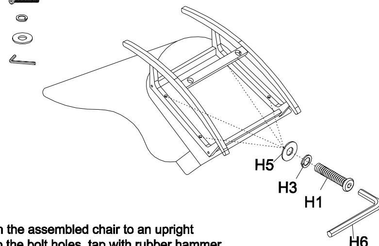
Step 3. Securely tighten all bolts, turn the assembled chair to an upright position. Insert wood plugs (H11) into the bolt holes, tap with rubber hammer or mallet until the wood plug edge are even with wood surface.
