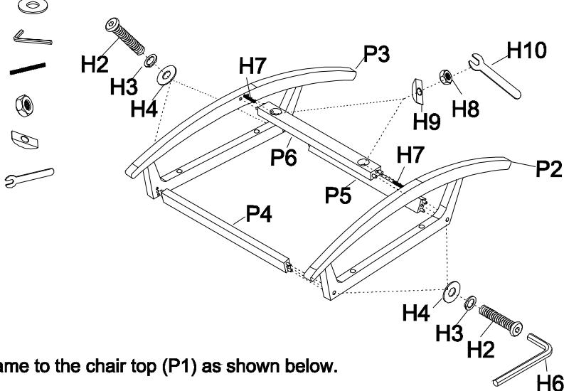
Step 2. Attach the assembled side frame to the chair top (P1) as shown below.
