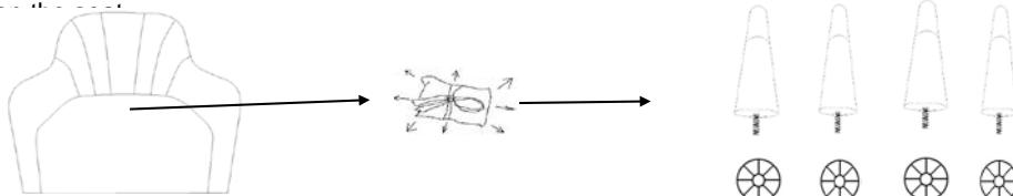
Step 2. Then turn the chair seat upside down. Place washers(H1) on legs(P1) and attach to chair seat by screwing clockwise into corresponding holes.
