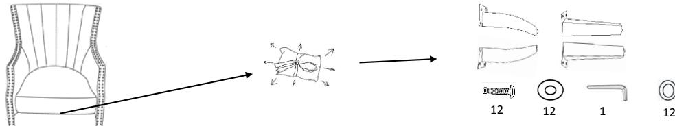
Step 2. Assemble the chair on a flat, soft surface such as carpet or cloth to prevent scratching. Place chair (P4) upside down onto a protective cloth. Using bolts (H2), lock washer (H4), flat washer (H1), connect legs (P1&P2&P3) to chair (P4). Tighten bolts (H2) with Allen Wrench (H3).
