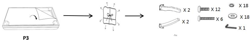
2. Using bolts (H2), lock washers (H3), flat washers (H4), connect backrest( P4 ) to seat frame( P3 ). Tighten bolts (H2) with Allen Wrench (H5).Affix the black cloth on bottom.
