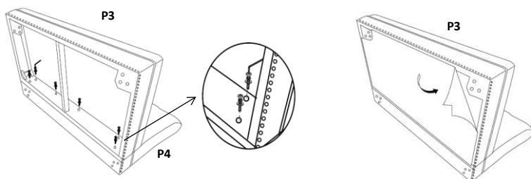
3.Using bolts (H1), lock washers (H3), flat washers (H4), connect legs(P1,P2) to seat frame (P3). Tighten bolts (H1) with Allen Wrench (H5).
