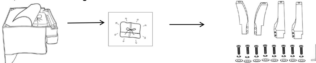
2. Attached the Legs to the seat frame by using Flat Washers (H3), Lock Washers(H2) and Bolts (H1). Securely tighten all bolts with Allen Wrench (H4).
