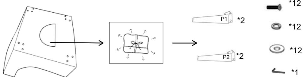
2. Attach the legs(P1,P2) to the seat frame by using Flat Washers (H3), Lock Washers(H2) and Bolts (H1). Securely tighten all bolts with Allen Wrench (H4).
