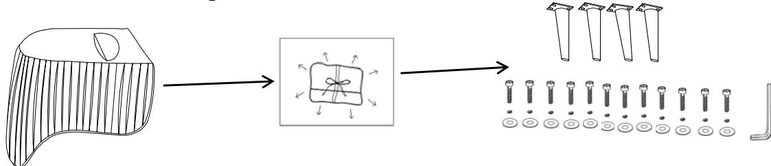
2. Attached the Legs to the seat frame by using Flat Washers (H3), Lock Washers(H2) and Bolts (H1). Securely tighten all bolts with Allen Wrench (H4).
