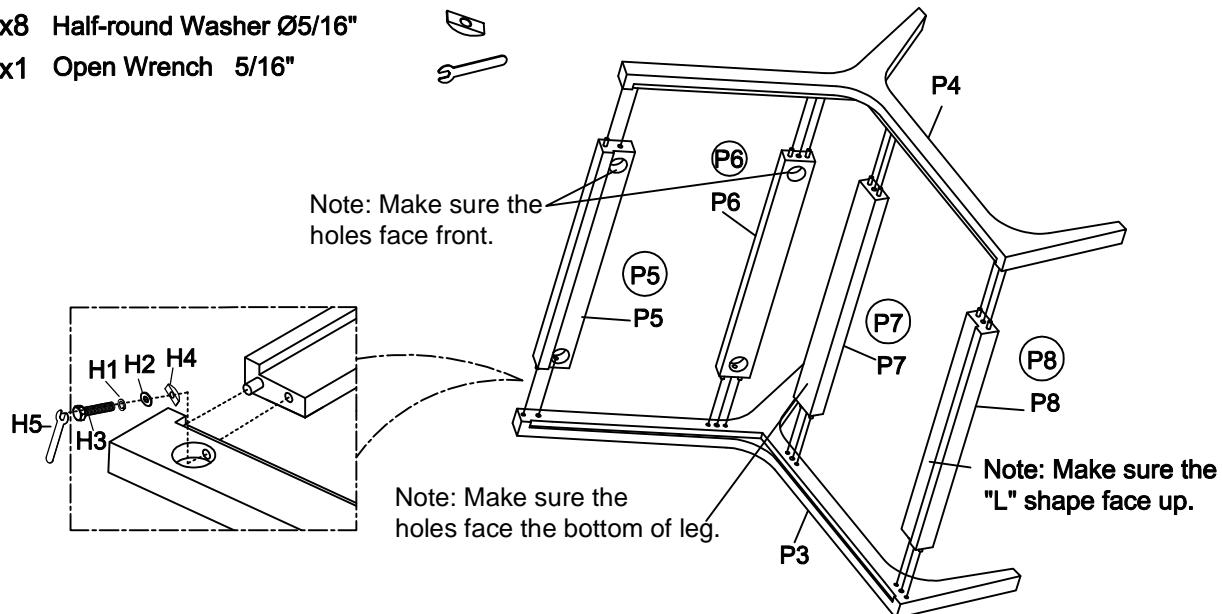
Step 2. Securely tighten all the bolts with open wrench (H5), but do not over tighten the bolts.
