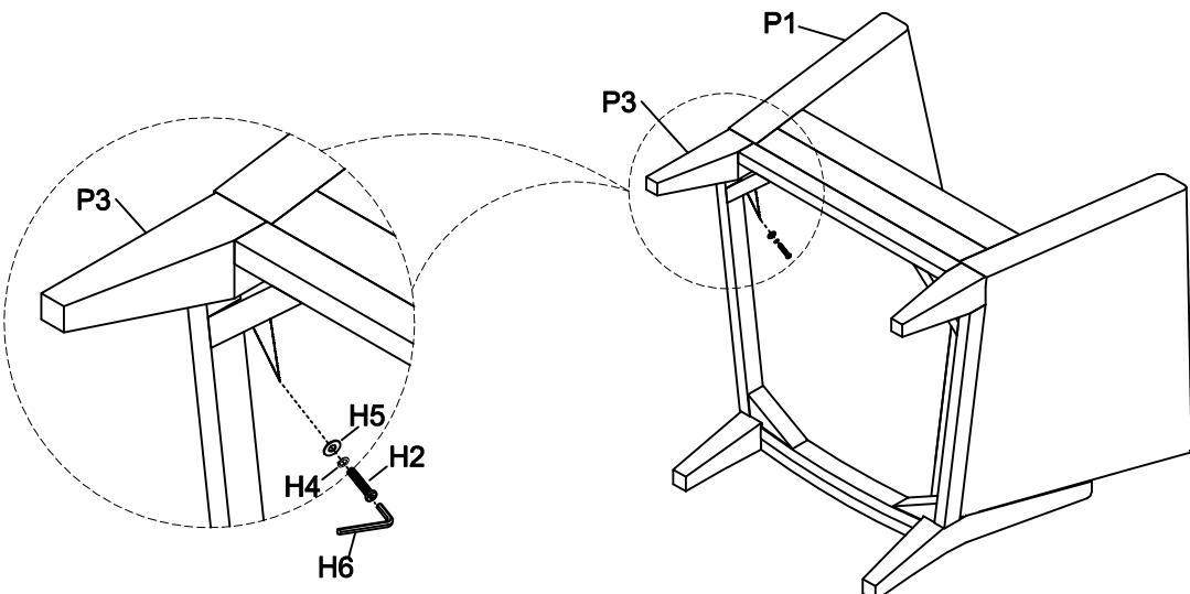
Step 3. Turn the assembled chair to an upright position. Make sure the chair is level and securely tighten all bolts with Allen wrench (H6). Assembly is complete. **Failure to follow these instructions may cause the bolts to misalign during assembly.**
