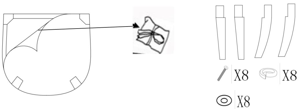
Step 2: Insert the front legs (A) and back legs (B) to seat frame , lock legs by using spring washer (E), flat washer(F), bolt(D), Then tighten the bolts with allen wrench (H).
