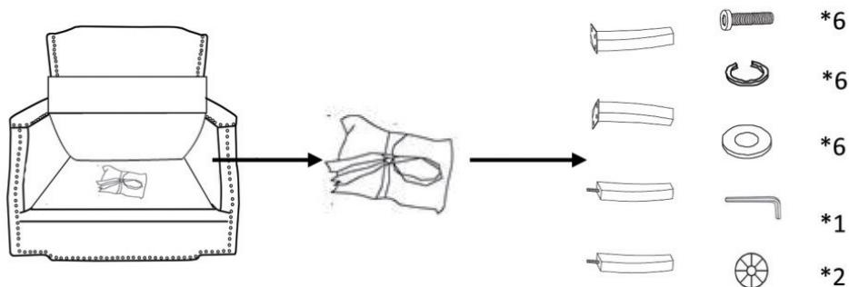
Step 2. Turn the chair upside down and lay on protective carpet. Screw in the back legs (P3) using Plastic Washer (H5) for each. Screw tight to the right angle.
