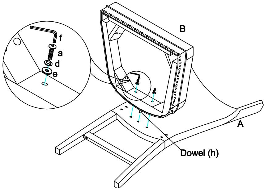
Step 2. Attach the seat cushion (B) to the leg of chair back (A) using bolts (b), lock washers (d) and flat washers (e). Loosely tighten the bolts with Allen wrench (f).
