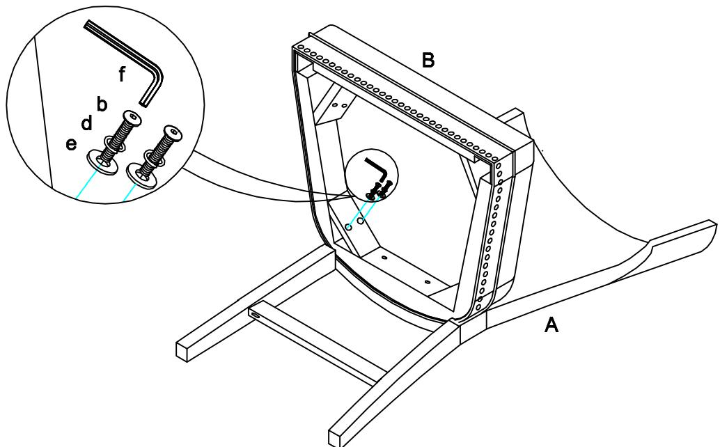
Step 3. Insert the right stretcher (D) to the leg of chair back (A) according to the label "R" at the hole in the leg of counter stool back and the front end of right stretcher (D). Loosely attach the front leg (F) to the bottom of seat cushion (B) and the stretcher (D) using bolts (c), lock washers (d), flat washers (e) and Allen wrench (f). Do not tighten the screws at this time.
