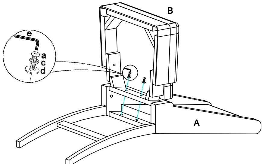
Step 2. Attach the seat cushion (B) to the leg of chair back (A) using bolts (a), lock washers (c) and flat washers (d). Loosely tighten the bolts with Allen wrench (e).
