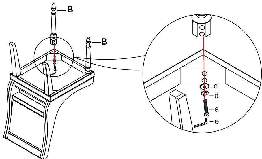
Step 3. Assembly is complete. Failure to follow these instructions may cause the bolts to misalign during assembly.
