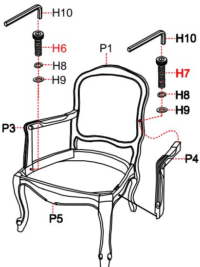
Step 4: Make sure the chair is level and securely tighten all bolts with Allen wrench (H6 & H10).
