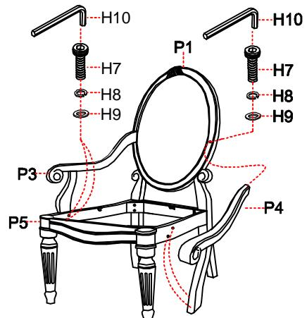
Step 4: Make sure the chair is level and securely tighten all bolts with Allen wrench (H6 & H10).
