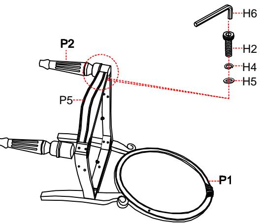
Step 3: Turn the assembled chair to an upright position. Attach the left arm (P3) and right arm (P4) to the seat frame (P5) and chair back (P1) as shown below.
