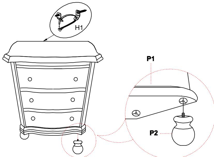
**ADDITIONAL NOTE ABOUT SAFETY:** BOLTS MAY LOOSEN DURING NORMAL EVERYDAY USE. THEY SHOULD BE PERIODICALLY INSPECTED AND RE-TIGHTENED TO PREVENT DAMAGE OR INJURY. ALWAYS CHECK TO BE SURE THAT ALL HARDWARE IS KEPT TIGHTENED.
