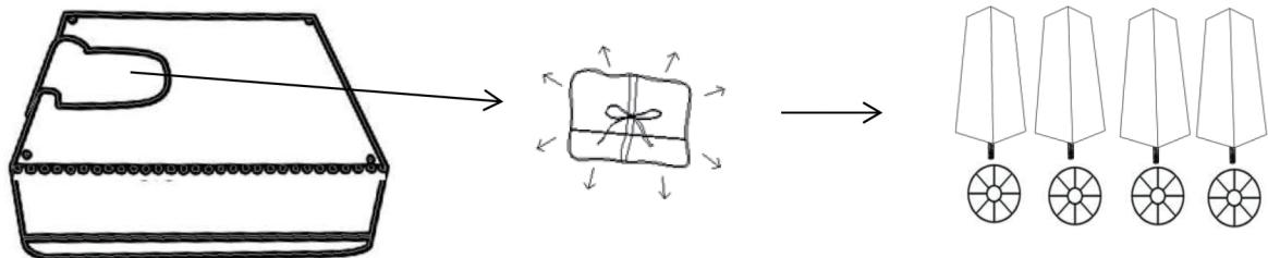
2. Place plastic washers(H1) on legs(P1) and attach to ottoman base by screwing clockwise into corresponding holes.
