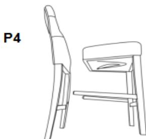
Step 5: Attach Cushion Seat (P5), Left and Right side Footrests (P1 & P2) to the Back Leg Frame (P4) using Allen Wrench (H4) with Lock Washer (H2), Flat Washer (H3) to secure the Cushion Seat and Screwdriver (H6) with Wood Screw (H5) to secure the Left and Right Footrest (P1 & P2) as shown below :
