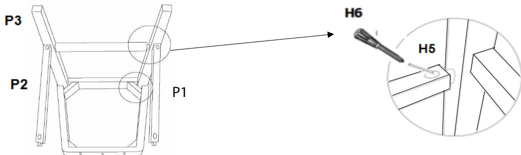
Step 4: Attach Step-3 assembled part to the Back Leg Frame (P4) as show below:
