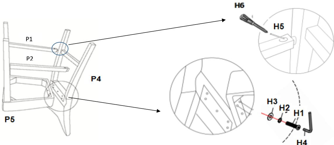
Step 6: Fully tighten all the bolts and screws with Allen Wrench (H4) and Screwdriver (H6) before turning the chair over and place it upright on a level surface. Assembly is completed.
