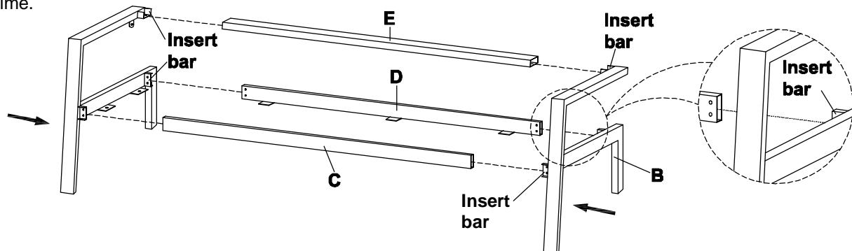
Step 2. Use  $\frac{1}{2}$ "L short Bolts (a) to attach left side metal frame (A) and right side metal frame (B) to front rail (C), back bottom rail (D) and back top rail (E). Securely tighten all bolts with Allen wrench (g).
