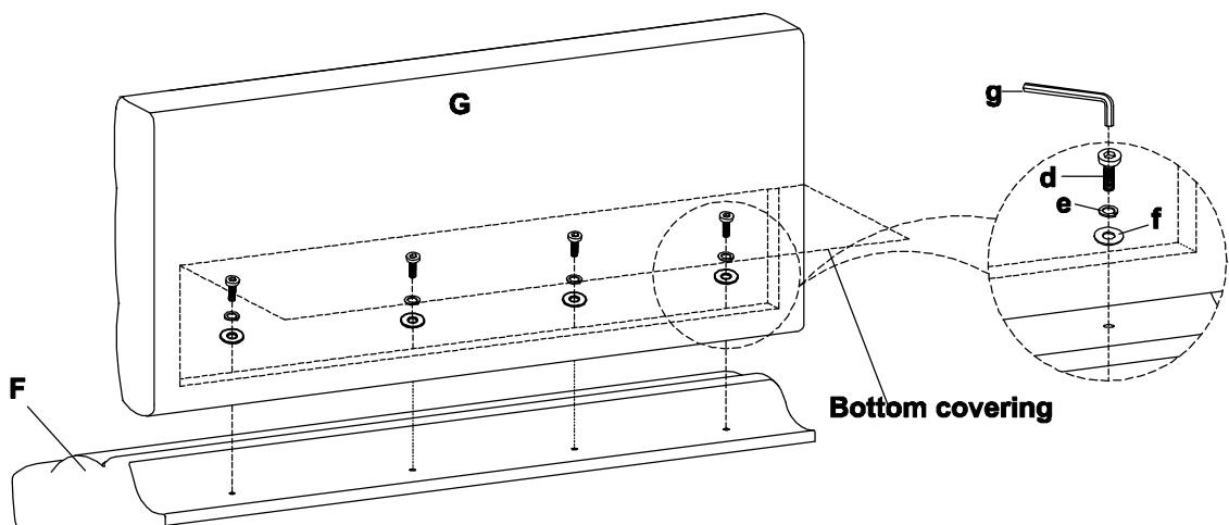
Step 4. Lift the assembled seat cushion (G) and back cushion (F) by two or more adults is recommended. Attach the bottom of seat cushion (G) on the left side metal frame (A) and right side metal frame (B) using 1" L medium bolts (b), lock washers (e) and flat washers (f). Loosely tighten all the bolts with Allen wrench (g).
