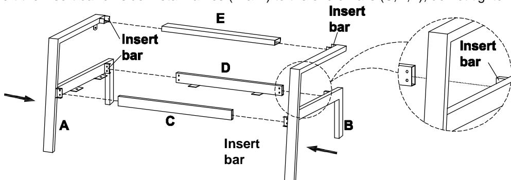
Step 2. Use  $\frac{1}{2}$ "L short Bolts (a) to attach left side metal frame (A) and right side metal frame (B) to front rail (C), back bottom rail (D) and back top rail (E). Securely tighten all bolts with Allen wrench (g).
