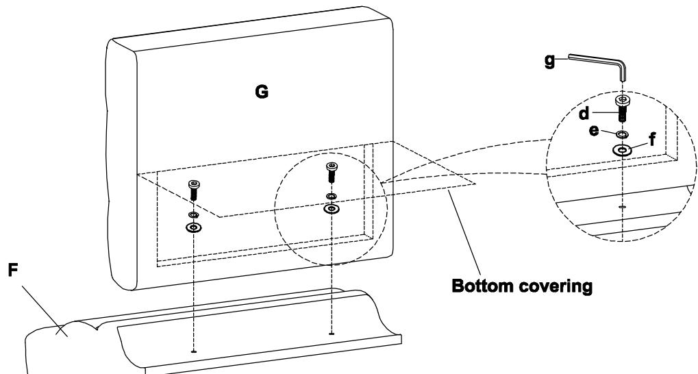
Step 4. Lift the assembled seat cushion (G) and back cushion (F) by two or more adults is recommended. Attach the bottom of seat cushion (G) on the left side metal frame (A) and right side metal frame (B) using 1" L medium bolts (b), lock washers (e) and flat washers (f). Loosely tighten all the bolts with Allen wrench (g).
