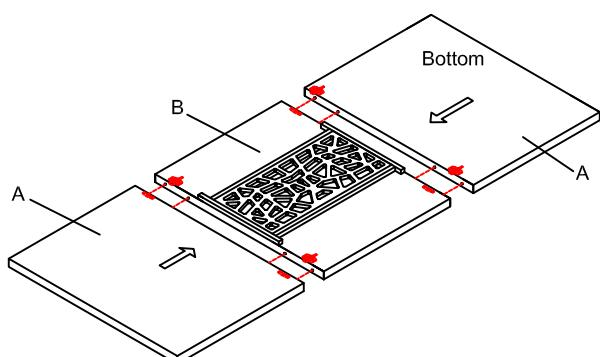
Step 2. Remove the protective panels on four corners as shown below.
