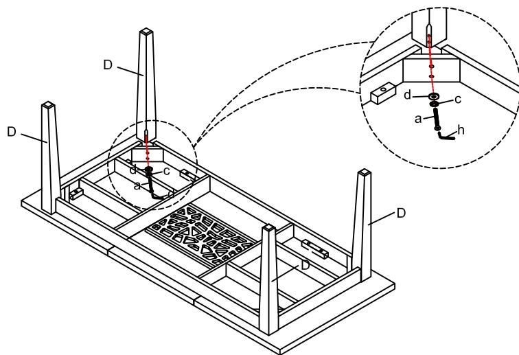
Step 5. Turn the assembled table to a upright position. Securely tighten all bolts by Allen wrench (d), but do not over tighten the bolts. Gently lay the glass top (E) on the table top.
