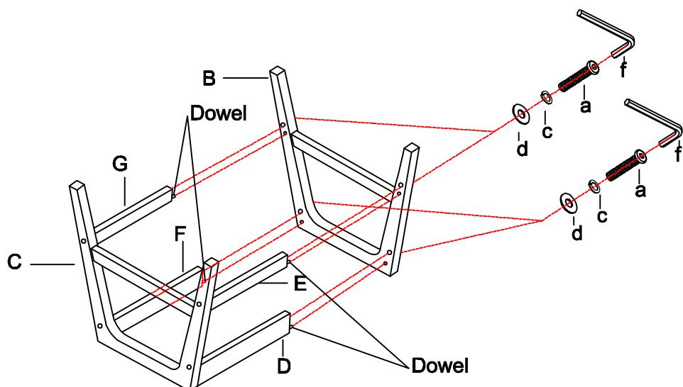
Step 3. Attach the assembled base to the bottom of the chair top (A) to using bolts (b), lock washers (c) and flat washers (e). Securely tighten all bolts by Allen wrench (f), but do not over tighten the bolts.
