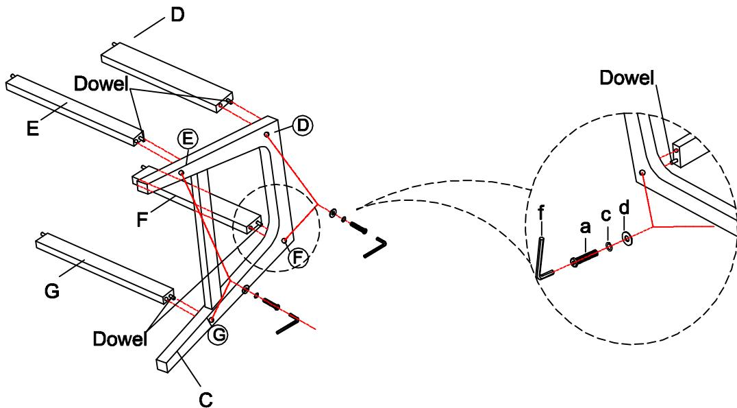
Step 2. Repeat the step 1 to attach left legs (B) to the rails and stretchers (D,E,F,G) using bolts (a), lock washers (c) and flat washers (d). Securely tighten all bolts by Allen wrench (f), but do not over tighten the bolts.
