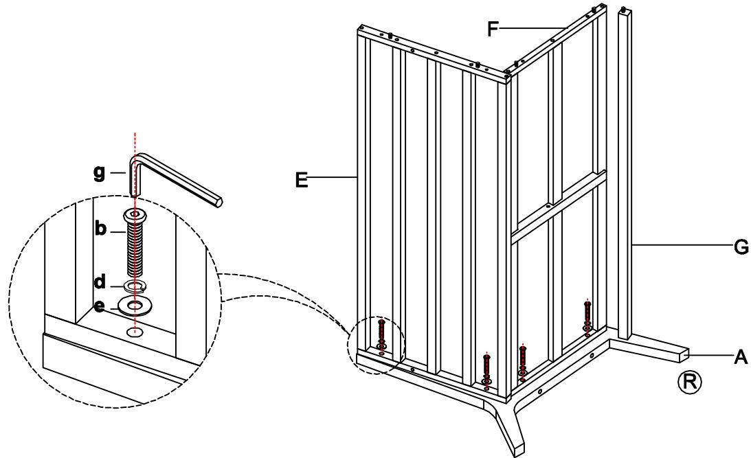
Step 2. Attach left leg (B) to the assembled stretcher (G), seat frame (F) and back frame (E) using bolts (b), lock washers (d) and flat washers (e) according to the label "L" on the left leg (B). Loosely tighten the bolts by Allen wrench (g) as shown below. Do not tight the screws at this time.
