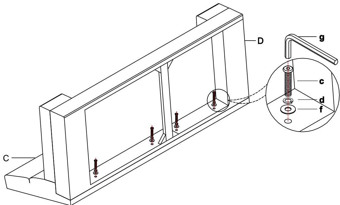
Step 5. Loosely attach the assembled back frame (E) to the assembled back cushion (C) using bolts (j), lock washers (d) and flat washers (e) as shown below . Loosely tighten the bolts by Allen wrench (g).
