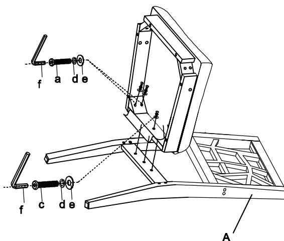
Step 2. Attach the front legs (C) to seat (A) using bolts (b), lock washers (d) and flat washers (e). Loosely tighten by Allen wrench (f).
