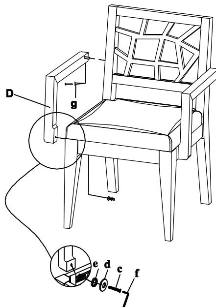
Step 4. Securely tighten all bolts by Allen wrench (f). Assembly is completed.
