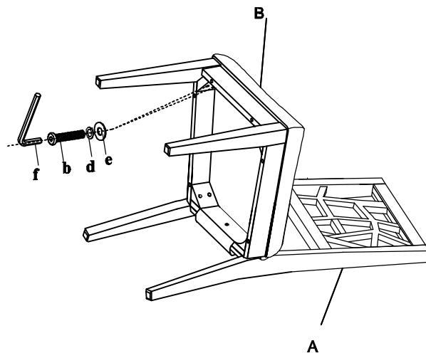
Step 3. 1) Attach the arms to the seat (B) by using bolts (c), locker washers (e), flat washers (d).
