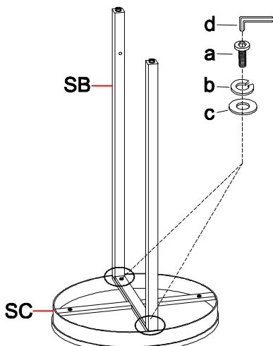
Step 2. Attach leg 1 (SA) to pedestal top (SC) with label "SB" using bolts (a), lock washers (b) and flat washers (c). Loosely tighten all bolts by Allen wrench (d) as shown below.
