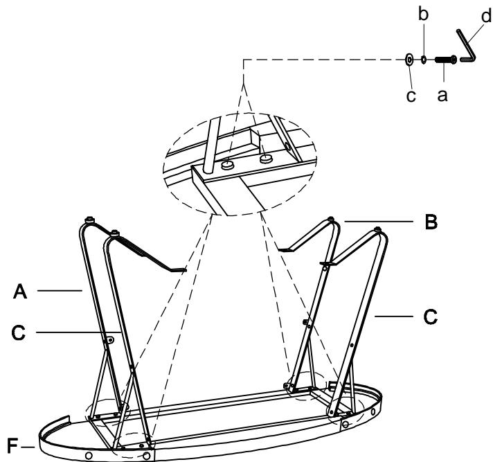
Step 2. Attach bottom shelf (G) to four legs (A,B,C) using bolts (a), lock washers (b) and flat washers (c) as shown. Loosely tighten by Allen wrench (d).
