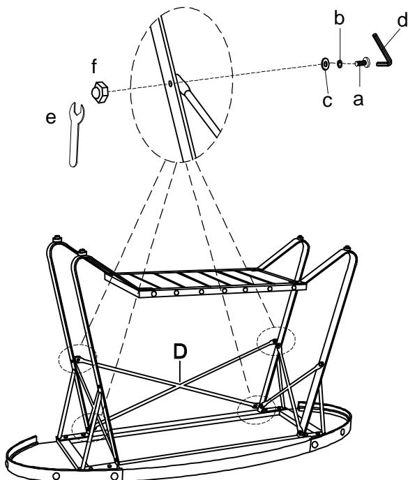
Step 5. Securely tighten all bolts and nuts, but do not over tighten the bolts or nuts. Turn the assembled table to an upright position, assembly is complete.
