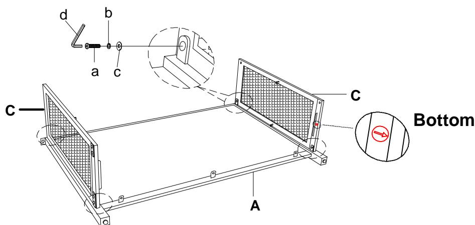
Step 2. Attach middle shelf (E) to back frame (A) and side panels (C) using bolts (e), lock washers (b) and flat washers (c). Loosely tighten by Allen wrench (d).
