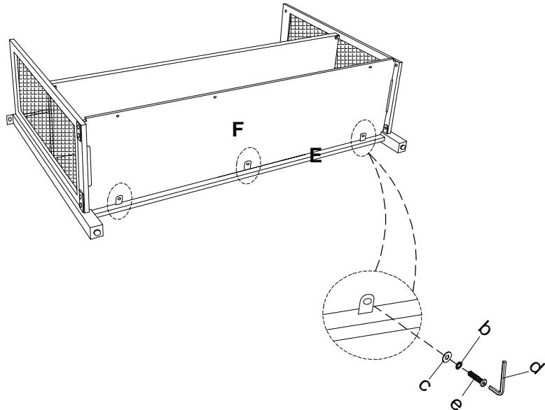
**Step 4. Attach the front frame (B) to bottom shelf (F) and side frames (C) using bolts (e & a), lock washers (b) and flat washers (c). Loosely tighten by Allen wrench (d).**
