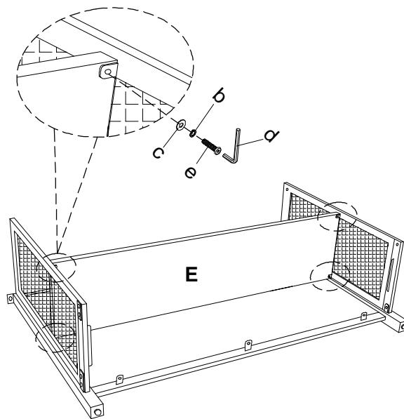
Step 3. Attach Bottom panel (F) to back frame (A) and side panels (C) using bolts (e), lock washers (b) and flat washers (c). Loosely tighten by Allen wrench (d).
