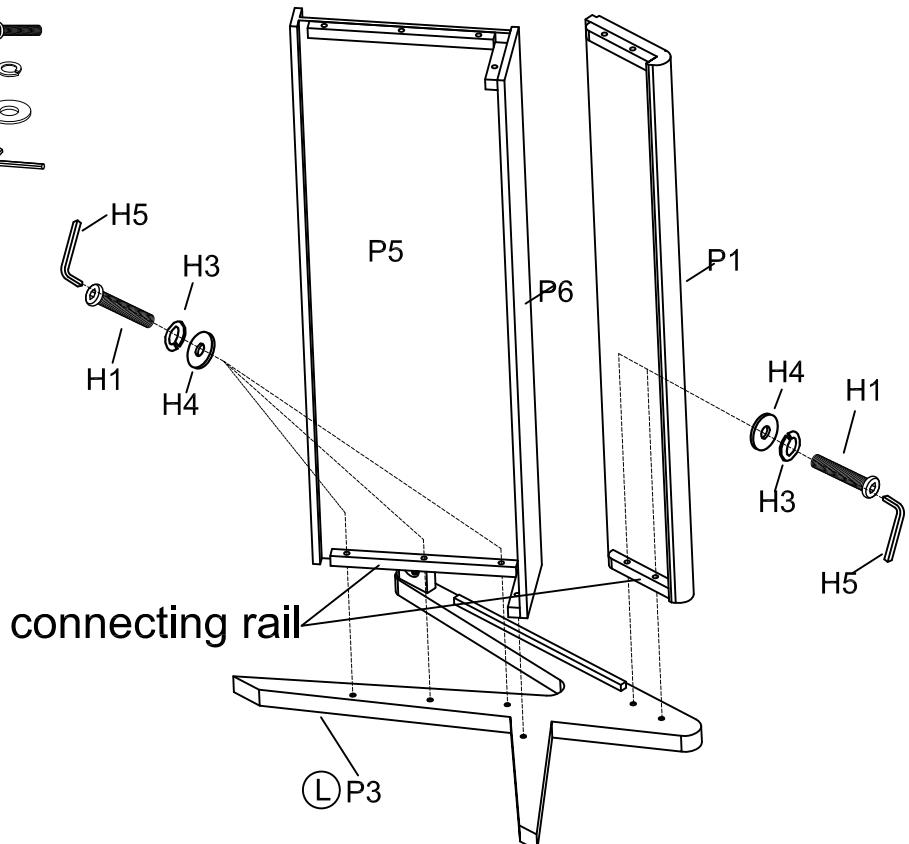
Step 4. Repeat Step 2 and Step 3 to attach the top frame 1 (P1) , the top frame 2 (P2) and the assembled shelf (P5 & P6) to the right leg (P4), see below diagram.
