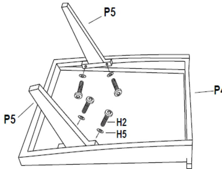
Step 2. Turn the seat (P2) over, and lock the armrest (P1) onto it with bolts(H2) and metal washers(H5).
