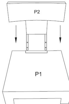
Step 2. Turn over the step1 part, fix the backrest and seat by using H1,H2,H5,H8, and securely tighten all bolts with Allen Wrench (H4) and Wrench(H7) ,then cover cap (H3) and (H6) on bolts
